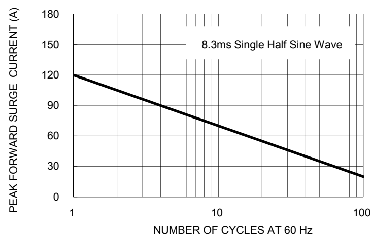
FIG. 2 MAXIMUM NON-REPETITIVE FORWARD SURGE CURRENT PER LEG
