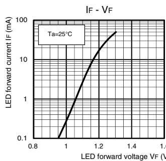
**Trigger LED forward current vs.
