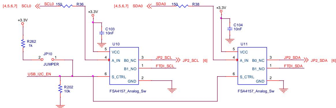
Figure 6.2. I<sup>2</sup>C MUX Circuits
