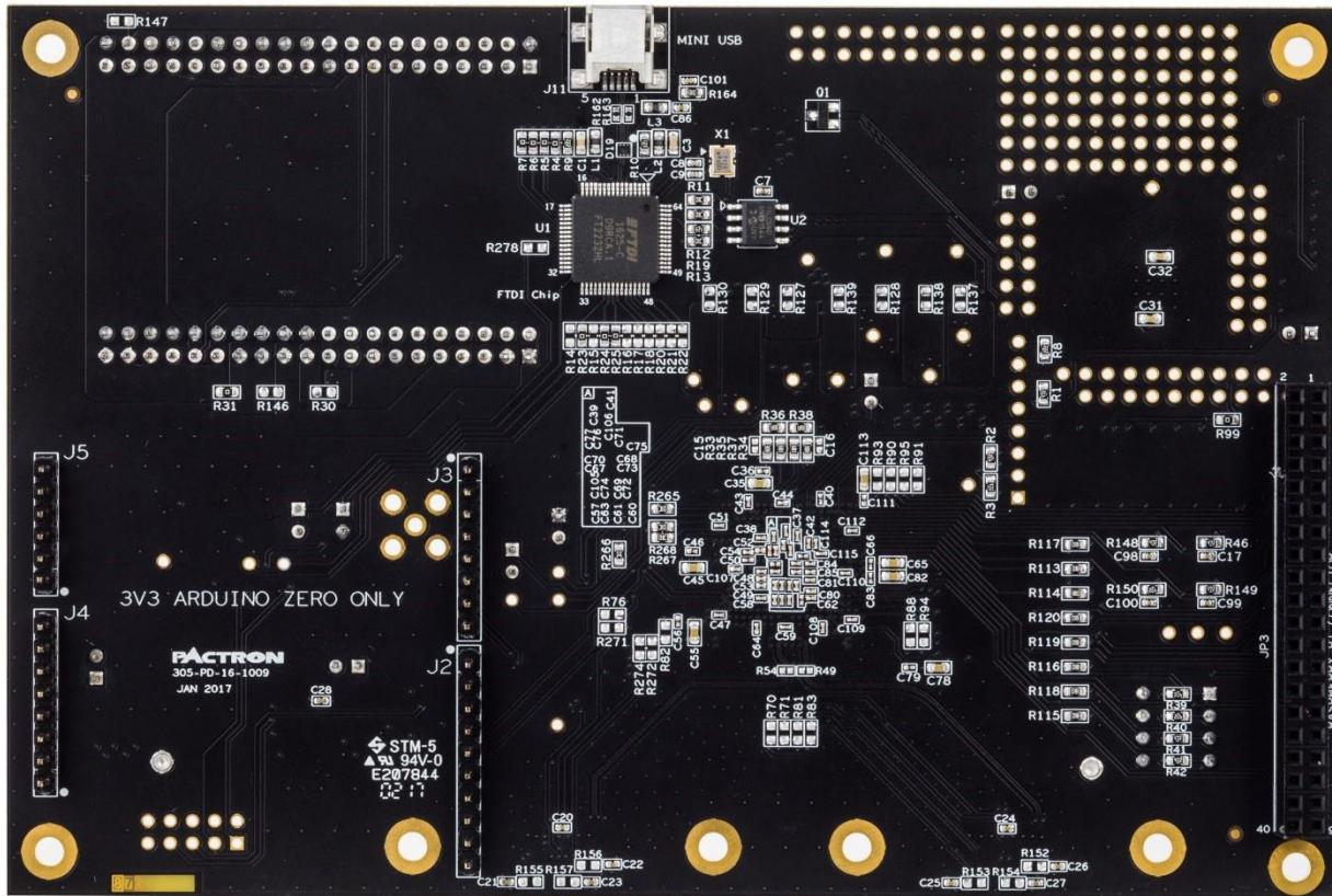
Figure 1.2. Bottom View of MachXO3-9400 Development Board
