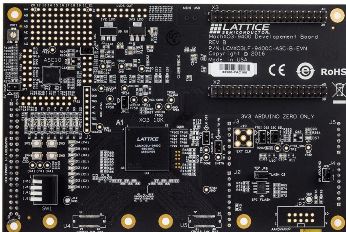
Figure 1.1. Top View of MachXO3-9400 Development Board
