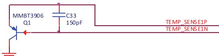
Figure 8.4. PNP Temperature Sensor Circuit
