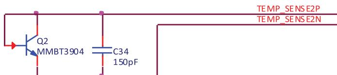
Figure 8.5. NPN Temperature Sensor Circuit
