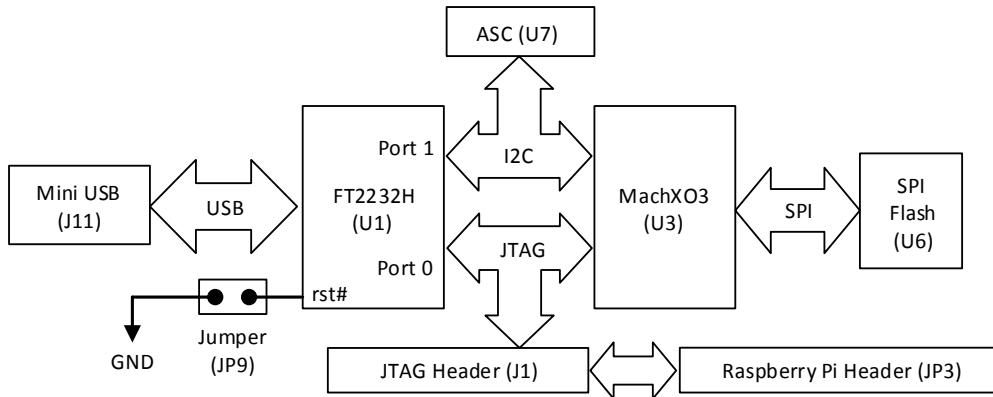
**Figure 3.1. JTAG/I<sup>2</sup>C Programming Architecture**
