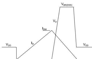
**Figure 18: Switching time waveform**
