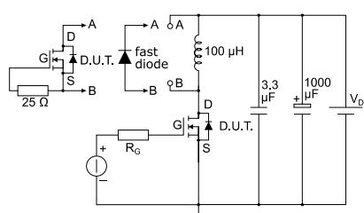
**Figure 16: Unclamped inductive load test circuit**
