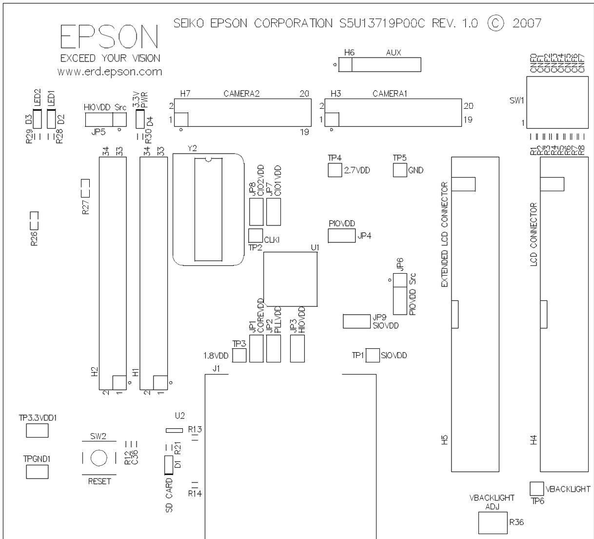
Figure 7-1: S5U13719P00C100 Board Layout - Top View
