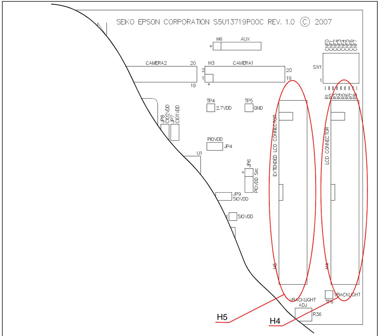
Figure 4-3: LCD Panel Connectors Locations (H4, H5)
