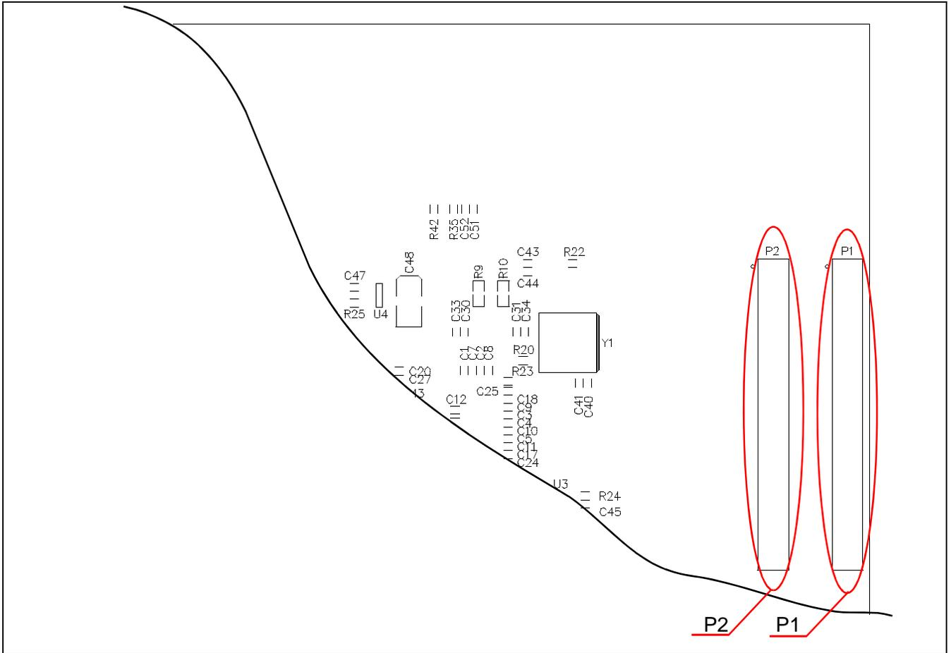
Figure 4-2: USB Adapter Connector Locations (P1 and P2 - Board Bottom)
