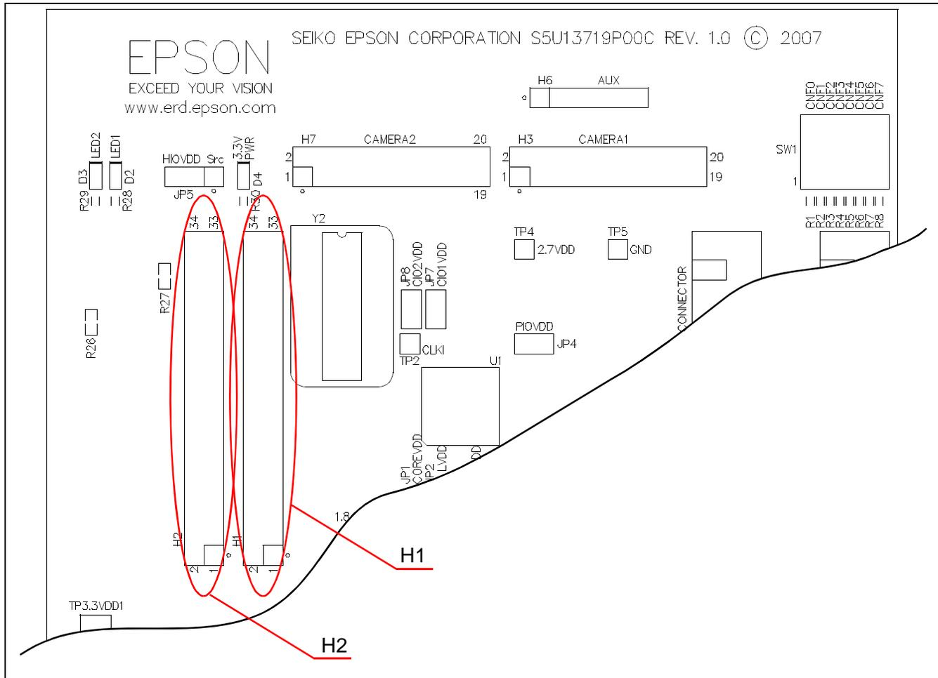
Figure 4-1: Host Bus Connector Location (H1 and H2)
