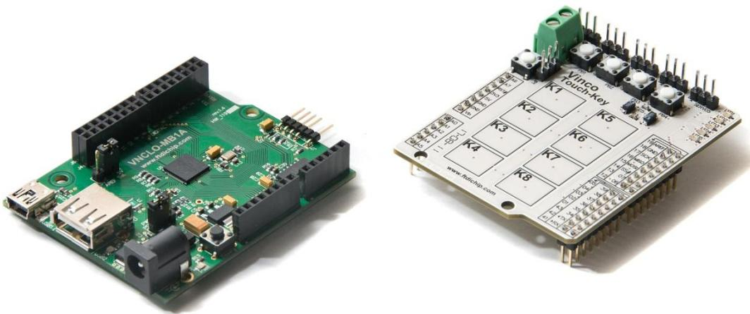
**Figure 1.1 – VINCO Development Module and the Touch-Key Shield**
