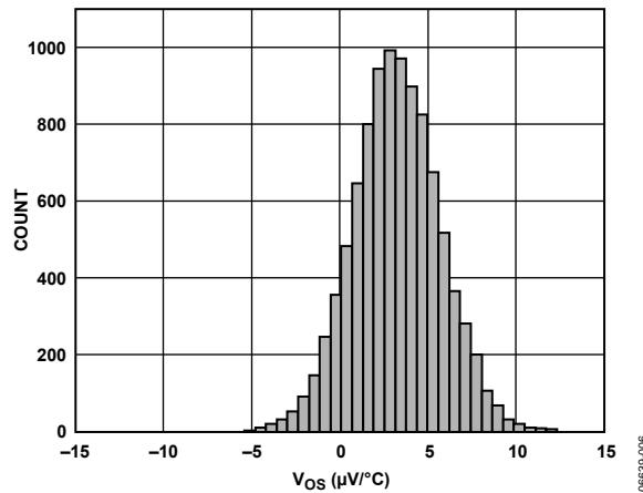
Figure 22. Offset Drift Distribution ( $V_{OS}$ ),
