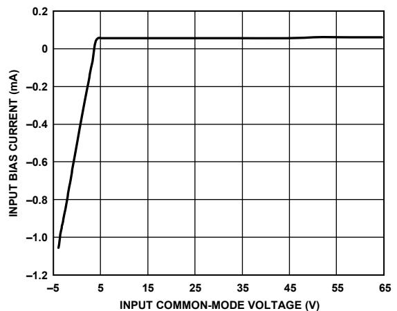
Figure 10. Input Bias Current vs. Input Common-Mode Voltage
