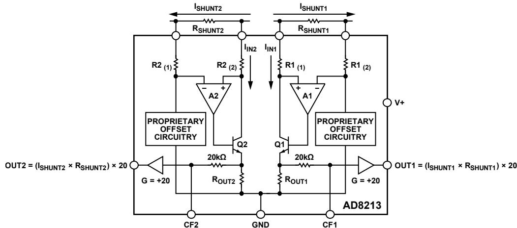
Figure 25. Simplified Schematic
