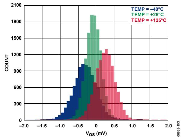
Figure 24. Offset Distribution ( $V_{OS}$ ),  $V_{CM} = 6 V$
