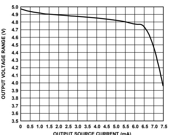
Figure 20. Output Voltage Range vs. Output Source Current Per Channel
