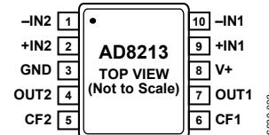
Figure 3. Pin Configuration
