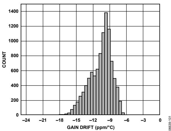
Figure 23. Gain Drift Distribution, Temperature Range =  $-40^\circ C$  to  $+125^\circ C$
