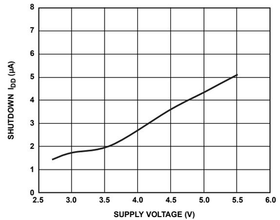
Figure 9. Shutdown Current vs. Supply Voltage
