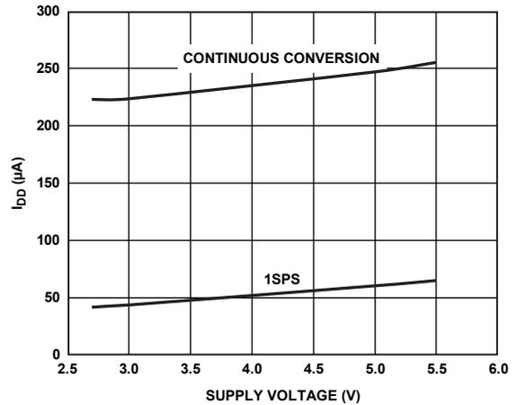
Figure 8. Average Operating Supply Current vs. Supply Voltage
