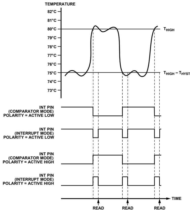
Figure 19. INT Output Temperature Response for T<sub>HIGH</sub> Overtemperature Events
