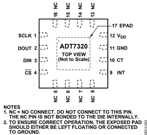
Figure 3. Pin Configuration
