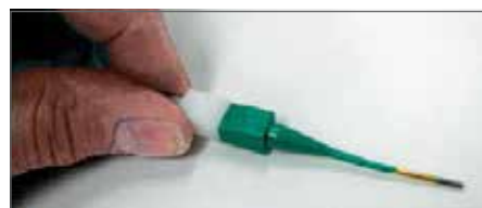
Plastic tool with contact in proper position.
