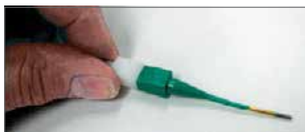
Plastic tool with contact in proper position.
