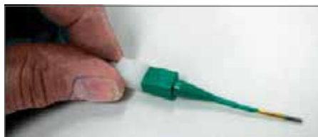
Plastic tool with contact in proper position.
