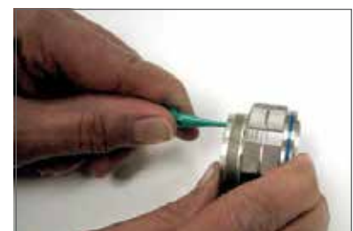
Plastic tool with contact in proper position.
