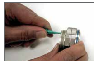
Plastic tool with contact in proper position.
