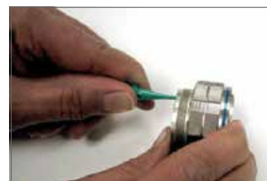
Plastic tool with contact in proper position.
