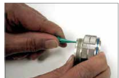
Plastic tool with contact in proper position.
