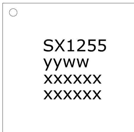
Figure 7-3: SX1255 Marking Diagram
