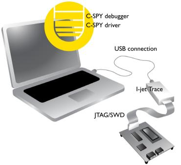
I-jet Trace connects to the target board via a JTAG or SWD connection, and to the host computer via the USB port.
