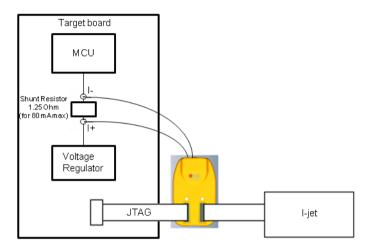
Based on this example, the dynamic range of the power probe would be from about 20 uA (80 mA/4096) to 80 mA.
