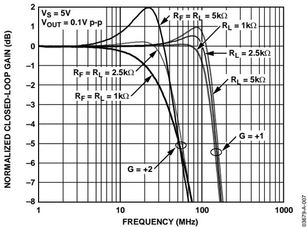
Figure 55. Frequency Response for Various Feedback/Load Resistances
