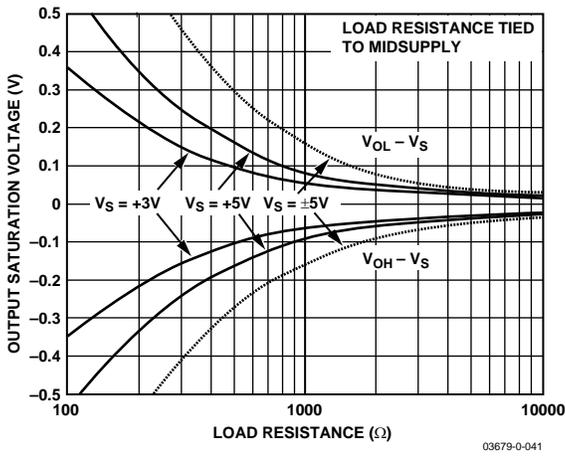
Figure 44. Output Saturation Voltage vs. Load Resistance
