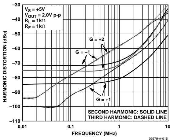
Figure 21. Harmonic Distortion vs. Frequency and Gain
