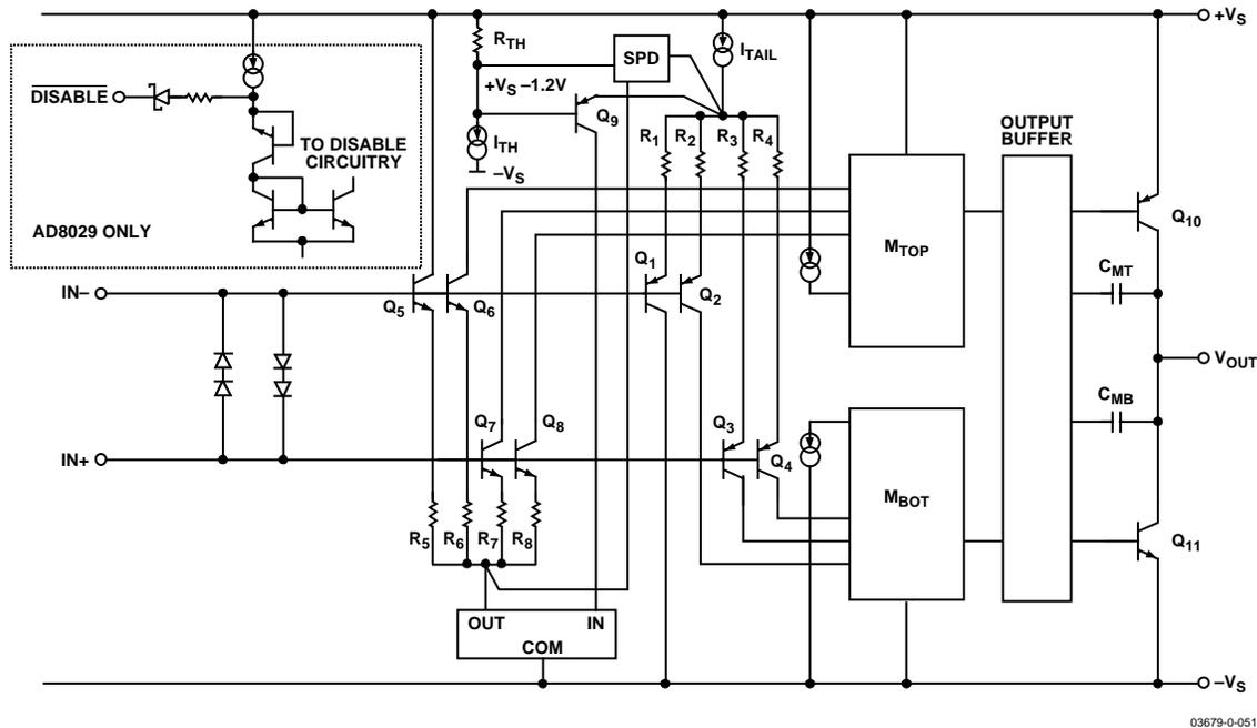
Figure 50. Simplified Schematic
