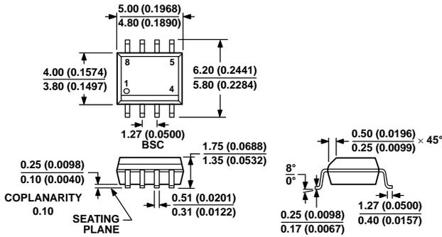
Figure 56. 8-Lead Standard Small Outline Package, Narrow Body [SOIC\_N] (R-8)
