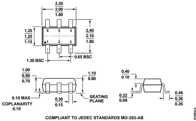
Figure 57. 6-Lead Plastic Surface-Mount Package [SC70] (KS-6)
