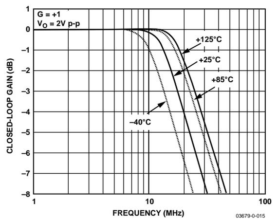
Figure 18. Large Signal Frequency Response vs. Temperature
