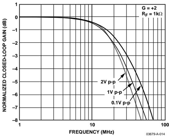
Figure 14. Frequency Response for Various Output Amplitudes
