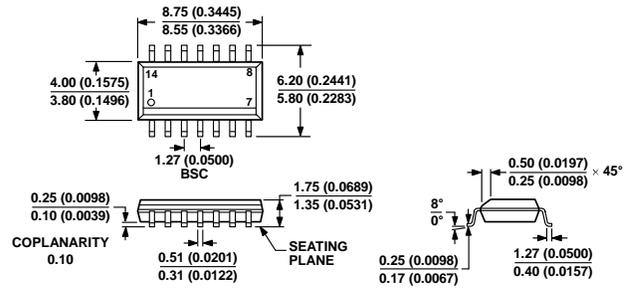
Figure 59. 14-Lead Standard Small Outline Package [SOIC\_N] (R-14)
