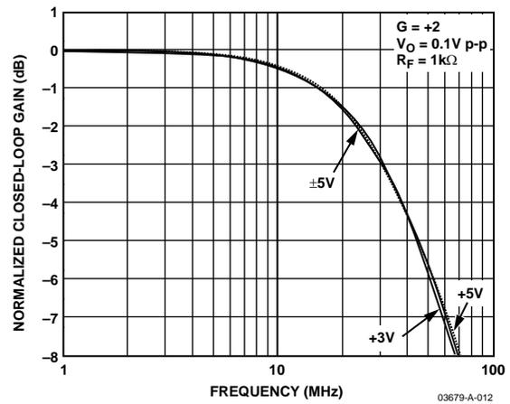
Figure 11. Small Signal Frequency Response for Various Supplies
