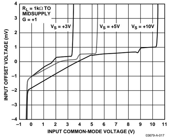
Figure 40. Input Offset Voltage vs. Input Common-Mode Voltage
