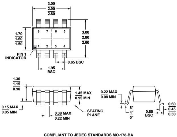
Figure 58. 8-Lead Small Outline Transistor Package [SOT-23] (RJ-8)
