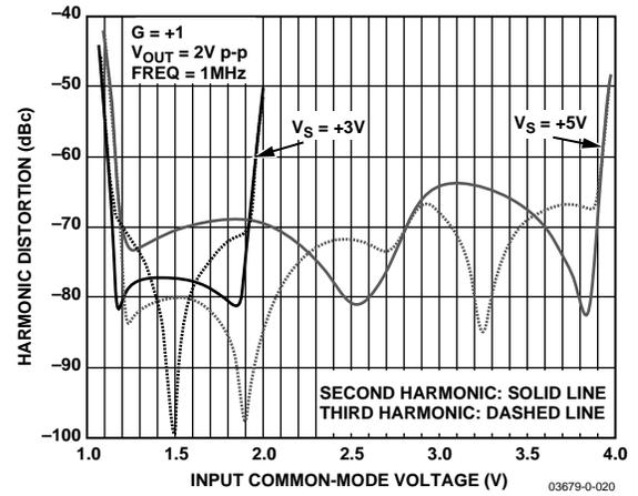
Figure 23. Harmonic Distortion vs. Input Common Mode Voltage
