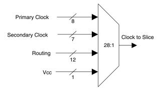
Figure 2-18. Slice0 through Slice2 Control Selection
