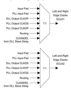
Figure 2-21. Sources of Edge Clock (Top Edge)
