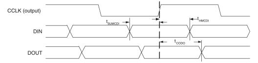
Figure 3-23. sysCONFIG Slave Serial Port Timing
