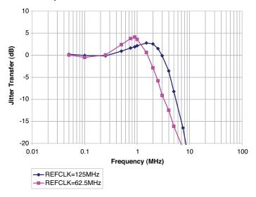
Figure 3-17. Jitter Transfer – 622 Mbps
