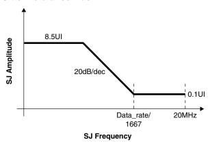
Note: The sinusoidal jitter tolerance is measured with at least 0.37Ulpp of Deterministic jitter (Dj) and the sum of Dj and Rj (random jitter) is at least 0.55Ulpp. Therefore, the sum of Dj, Rj and Sj (sinusoidal jitter) is at least 0.65Ulpp (Dj = 0.37, Rj = 0.18, Sj = 0.1).
