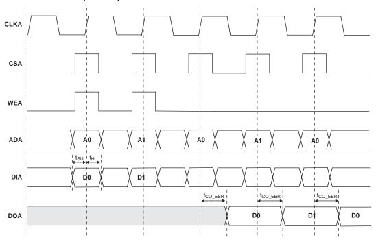
Note: Input data and address are registered at the positive edge of the clock and output data appears after the positive edge of the clock.
