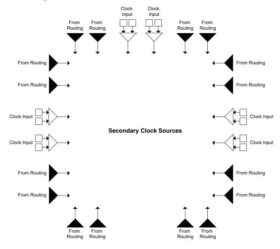
Note: Clock inputs can be configured in differential or single-ended mode.
