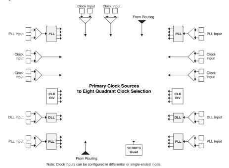
Figure 2-11. Primary Clock Sources for LatticeECP3-70, -95, -150
