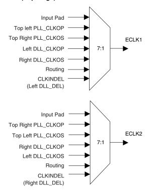
The edge clocks have low injection delay and low skew. They are used to clock the I/O registers and thus are ideal for creating I/O interfaces with a single clock signal and a wide data bus. They are also used for DDR Memory or Generic DDR interfaces.
