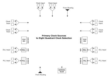
Note: Clock inputs can be configured in differential or single-ended mode.
