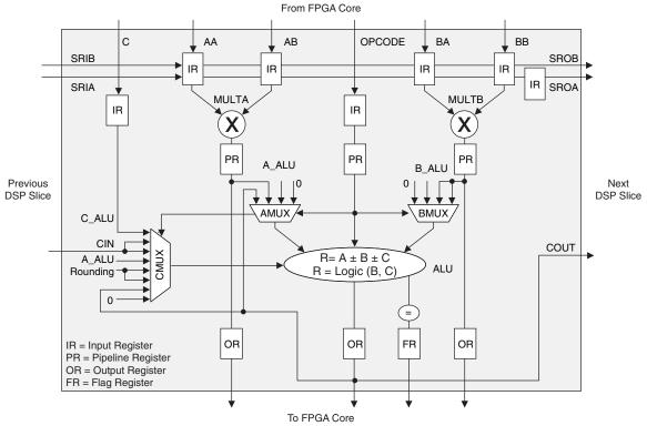
Note: A\_ALU, B\_ALU and C\_ALU are internal signals generated by combining bits from AA, AB, BA BB and C inputs. See TN1182, LatticeECP3 sysDSP Usage Guide, for further information.
