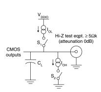
$\mathbf{C_{l}}$  including probe and jig capacitance, 3pF max.  $\mathbf{S_{l}}$  - open,  $\mathbf{S_{2}}$  - closed for  $\mathbf{V_{OH}}$  measurement.  $\mathbf{S_{l}}$  - closed,  $\mathbf{S_{2}}$  - open for  $\mathbf{V_{OL}}$  measurement.
