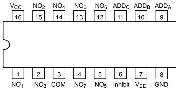
Figure 1. Pin Connection (Top View)
