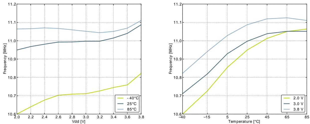
**Figure 3.24. Calibrated HFRCO 14 MHz Band Frequency vs Supply Voltage and Temperature**
