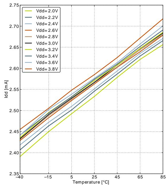
**Figure 3.4. EMO Current consumption while executing prime number calculation code from flash with HFRCO running at 11MHz**
