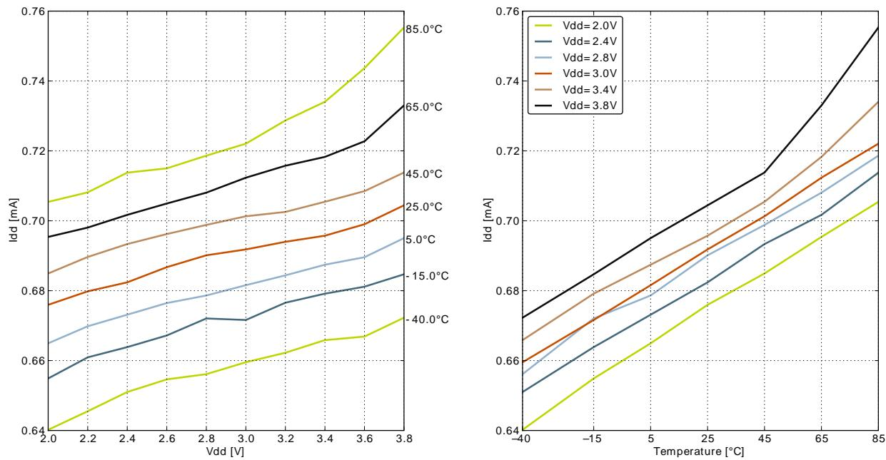
**Figure 3.9. EM1 Current consumption with all peripheral clocks disabled and HFRCO running at 11MHz**
