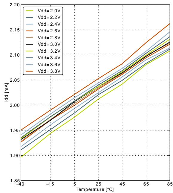
**Figure 3.5. EM0 Current consumption while executing prime number calculation code from flash with HFRCO running at 7MHz**
