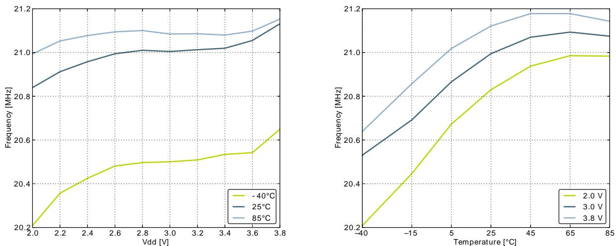
**Figure 3.26. Calibrated HFRCO 28 MHz Band Frequency vs Supply Voltage and Temperature**
