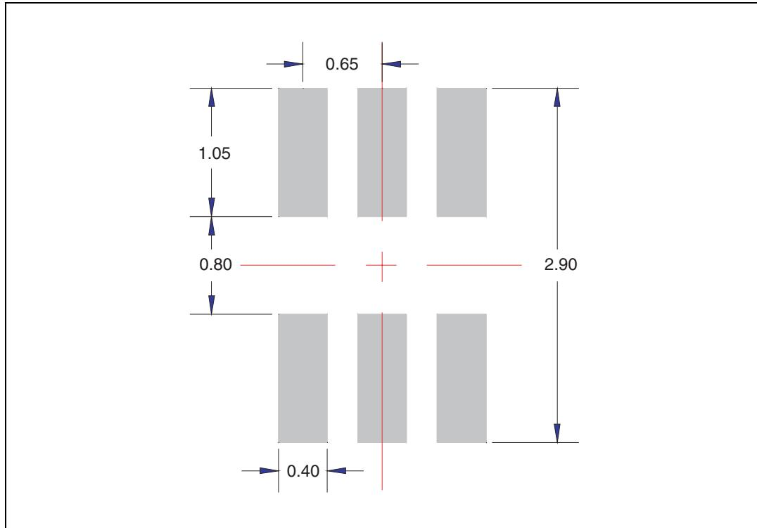
Figure 30. SC70-6 (or SOT323-6) package mechanical data
