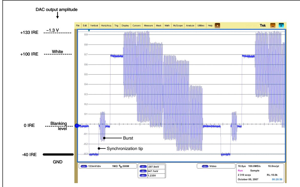
With its internal DC shift, the TSH122 can drive a video signal from the DAC output as low as 0 V (bottom of the synchronization tip at 0 V - see [Figure 14](#)).
