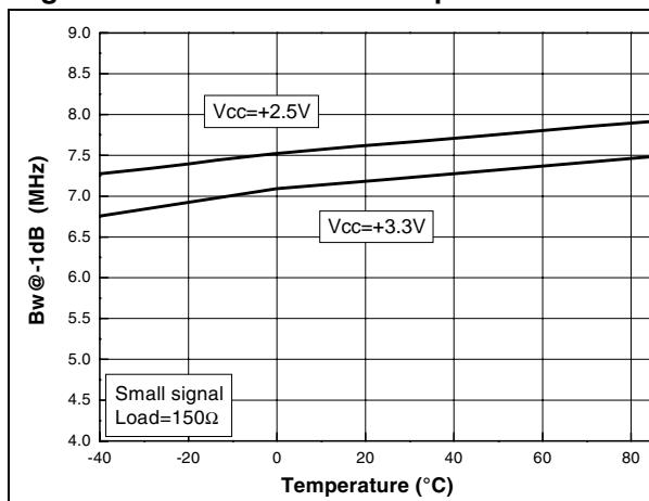
Figure 18. Attenuation vs. temperature
