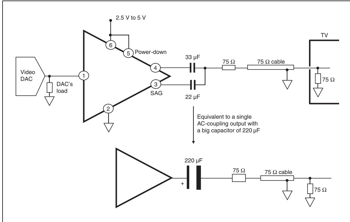
**Figure 27. Schematic diagram without output capacitor**
