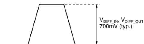
Figure 1b. Differential Voltage Swing
