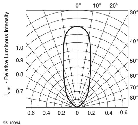
Figure 3. Rel. Luminous Intensity vs. Angular Displacement
