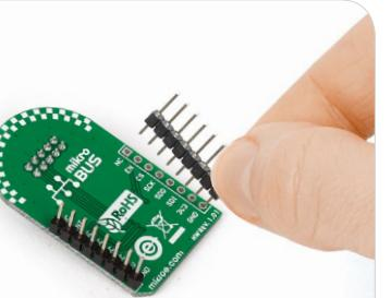
Turn the board upside down so that the bottom side is facing you upwards. Place shorter pins of the header into the appropriate soldering pads.
