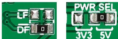
Counter click has two SMD jumpers [zero ohm resistor]. One lets you switch between a 3.3V or a 5V power supply. The other is for setting the interrupt as LFLAG [open drain latched output] or DFLAG [push-pull output].
