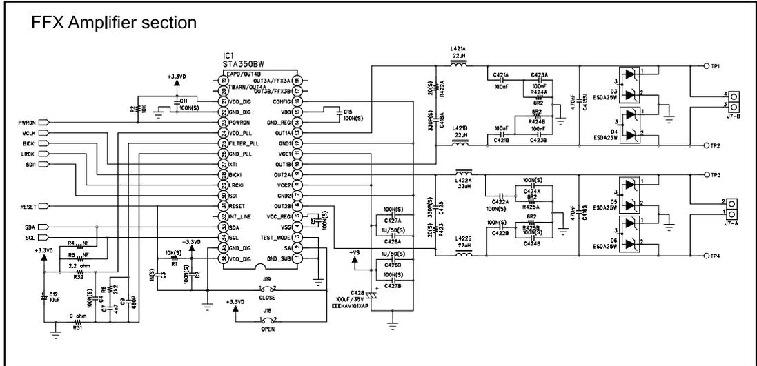
Figure 2: Schematic diagram (2 of 3)
