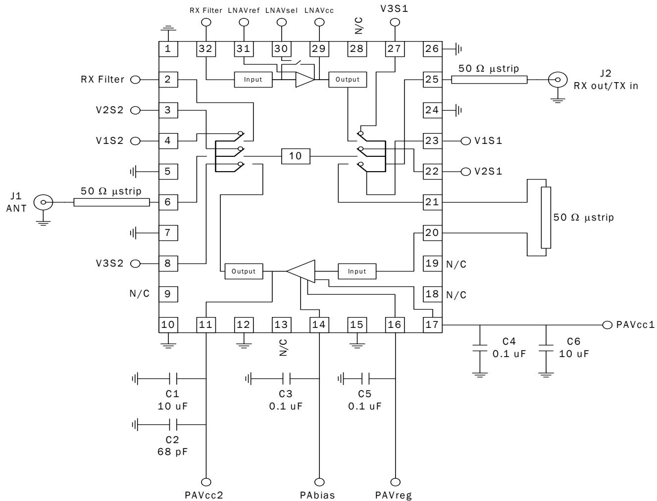
Note: 1. If extra isolation is needed between Tx and Rx path, the filter can be used otherwise for  $\leq 50$ dB isolation, 50Ω micro-strip should be okay.
