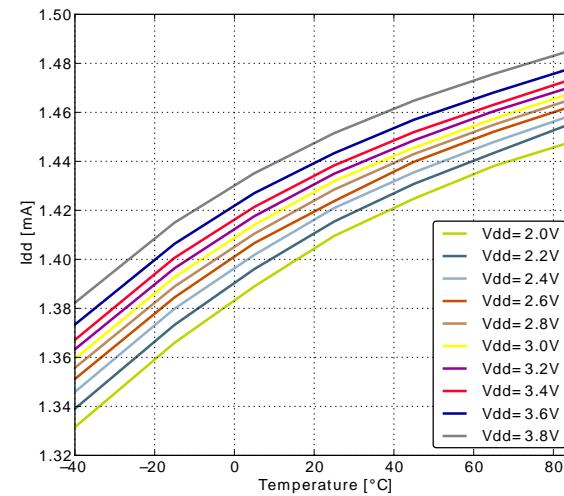
**Figure 3.10. EM1 Current consumption with all peripheral clocks disabled and HFRCO running at 14MHz**
