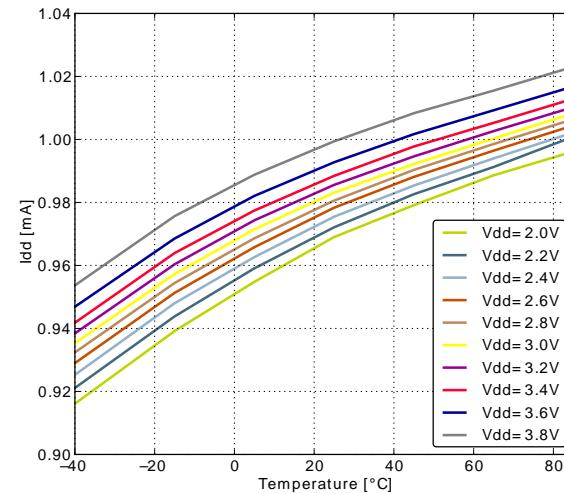
**Figure 3.11. EM1 Current consumption with all peripheral clocks disabled and HFRCO running at 11MHz**
