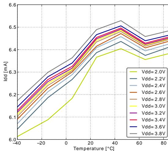
**Figure 3.3. EMO Current consumption while executing prime number calculation code from flash with HFRCO running at 21MHz**
