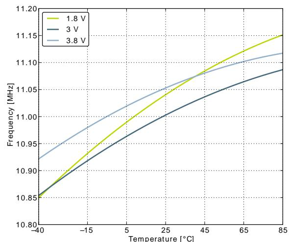
**Figure 3.25. Calibrated HFRCO 14 MHz Band Frequency vs Temperature and Supply Voltage**
