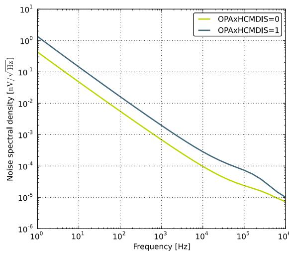
**Figure 3.40. OPAMP Voltage Noise Spectral Density (Non-Unity Gain)**
