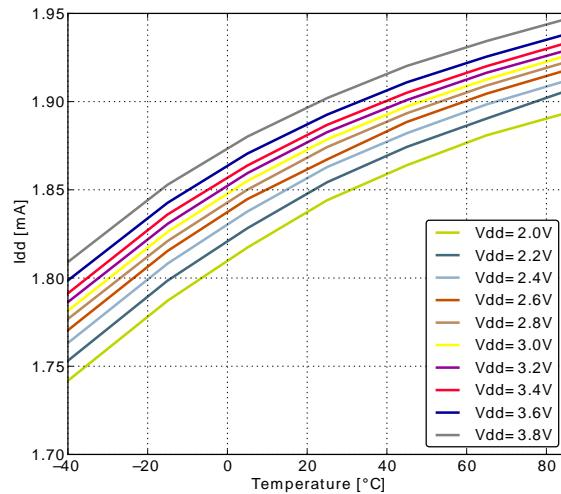
**Figure 3.9. EM1 Current consumption with all peripheral clocks disabled and HFRCO running at 21MHz**
