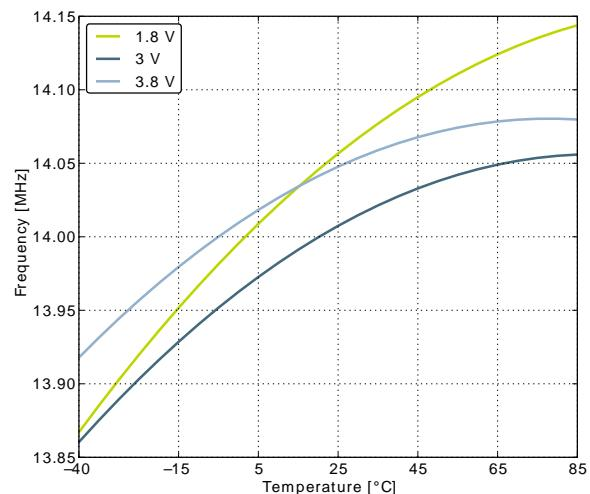
**Figure 3.26. Calibrated HFRCO 21 MHz Band Frequency vs Temperature and Supply Voltage**
