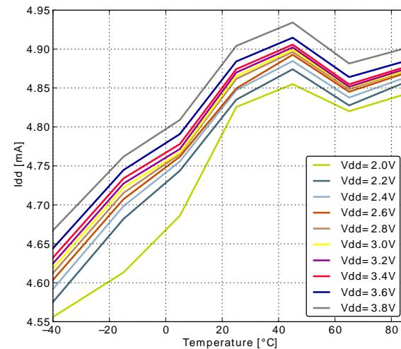
**Figure 3.4. EMO Current consumption while executing prime number calculation code from flash with HFRCO running at 14MHz**
