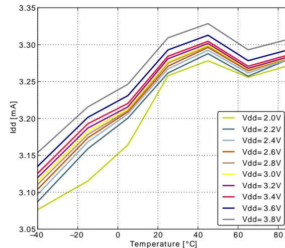
**Figure 3.5. EMO Current consumption while executing prime number calculation code from flash with HFRCO running at 11MHz**
