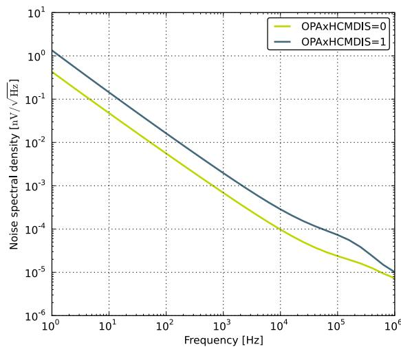
**Figure 3.40. OPAMP Voltage Noise Spectral Density (Non-Unity Gain)**
