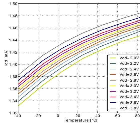
**Figure 3.10. EM1 Current consumption with all peripheral clocks disabled and HFRCO running at 14MHz**
