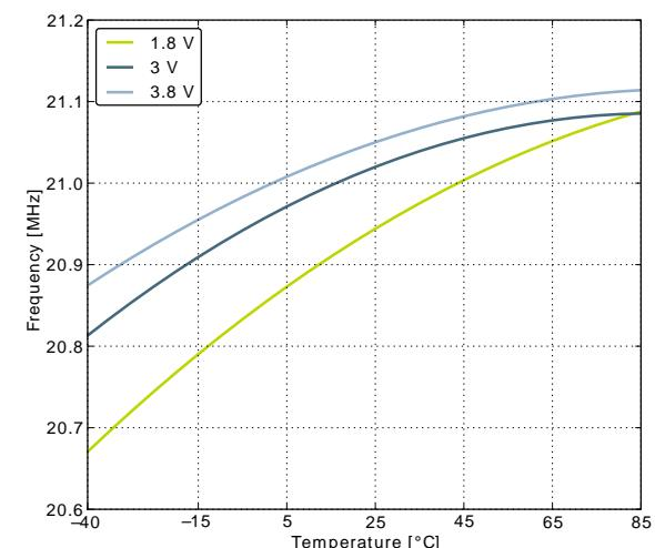
**Figure 3.27. Calibrated HFRCO 28 MHz Band Frequency vs Temperature and Supply Voltage**
