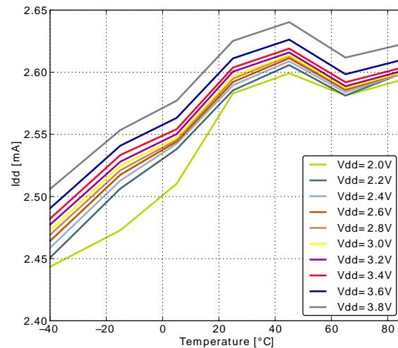
**Figure 3.6. EMO Current consumption while executing prime number calculation code from flash with HFRCO running at 7MHz**
