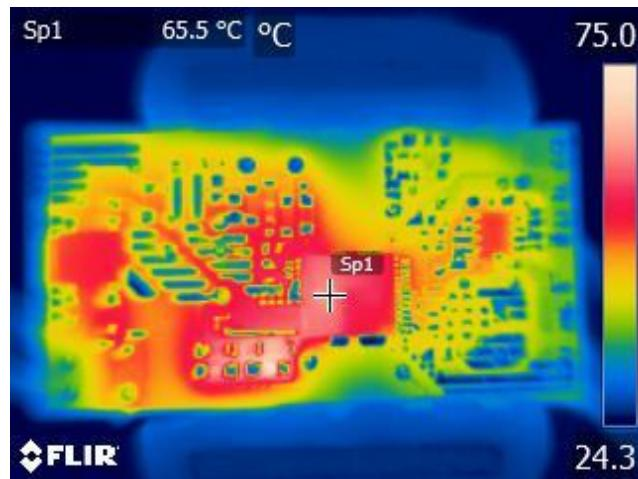
**Figure 19** – InnoSwitch3-EP Side. 90 VAC, Full Load.
