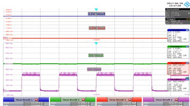
**Figure 27** – 0 A – 0.3 A, 5 V Load Step Transient Response, 265 VAC.
