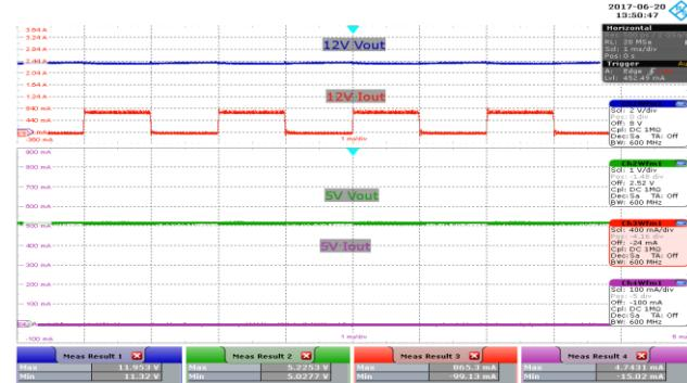
**Figure 25** – 0 A – 0.7 A, 12 V Load Step Transient Response, 265 VAC.
