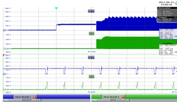
**Figure 30** – Drain Voltage and Current Waveforms.
