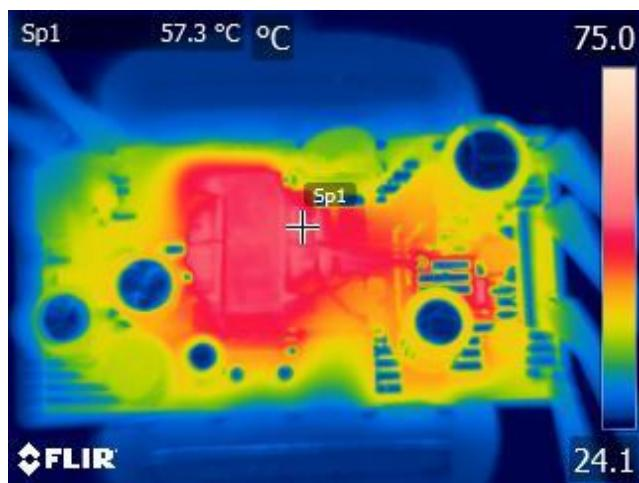
**Figure 20** – Transformer Side. 265 VAC, Full Load.
