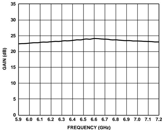
Figure 24. Gain vs. Frequency, BAND = 0 V
