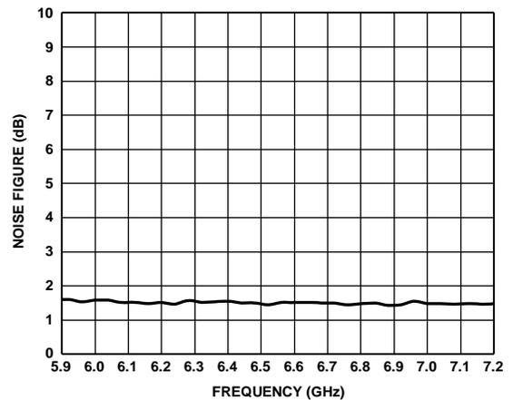
Figure 26. Noise Figure vs. Frequency, BAND = 0 V
