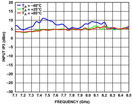
Figure 19. Input IP3 vs. Frequency for Various Temperatures
