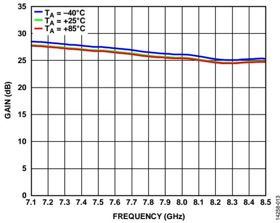
Figure 13. Gain vs. Frequency for Various Temperatures
