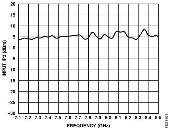
Figure 29. Input IP3 vs. Frequency, BAND = 1.8 V
