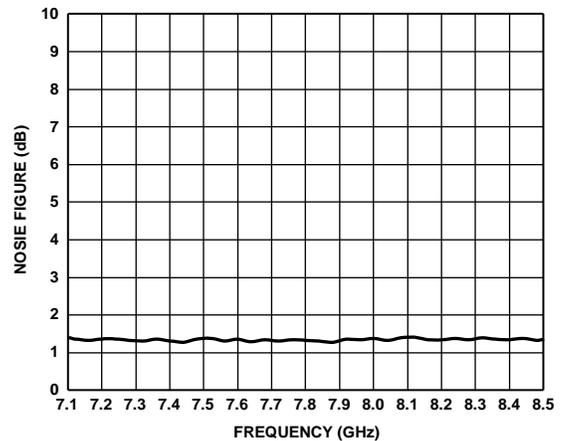
Figure 27. Noise Figure vs. Frequency, BAND = 1.8 V
