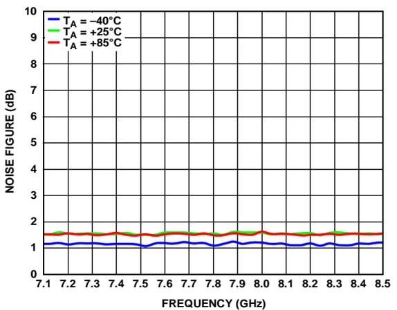
Figure 15. Noise Figure vs. Frequency for Various Temperatures
