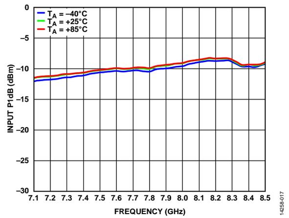
Figure 17. Input P1dB vs. Frequency for Various Temperatures
