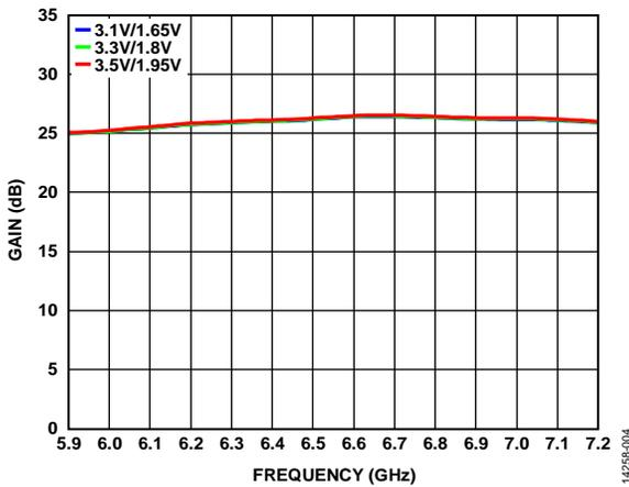
Figure 4. Gain vs. Frequency for Various Supply Voltages
