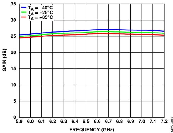
Figure 3. Gain vs. Frequency for Various Temperatures
