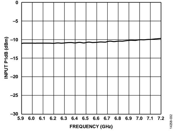
Figure 30. Input P1dB vs. Frequency, BAND = 0 V
