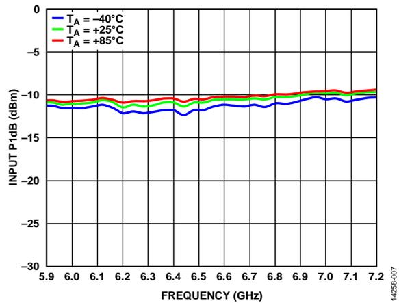
Figure 7. Input P1dB vs. Frequency for Various Temperatures
