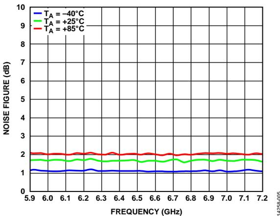
Figure 5. Noise Figure vs. Frequency for Various Temperatures
