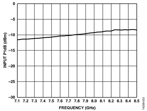
Figure 31. Input P1dB vs. Frequency, BAND = 1.8 V
