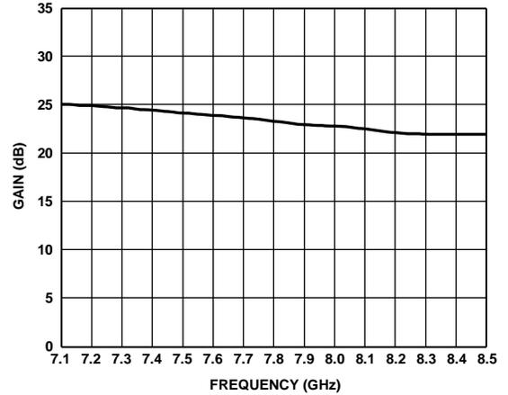
Figure 25. Gain vs. Frequency, BAND = 1.8 V
