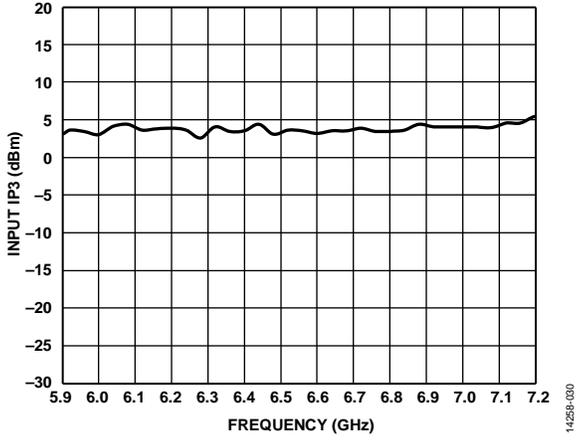
Figure 28. Input IP3 vs. Frequency, BAND = 0 V
