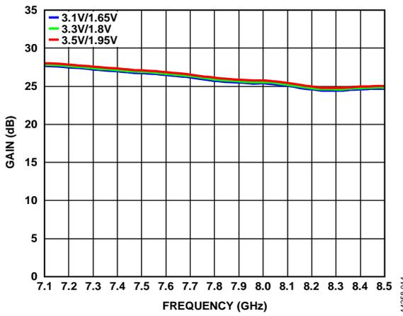
Figure 14. Gain vs. Frequency for Various Supply Voltages
