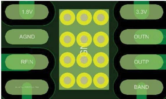
Figure 23. Evaluation Board Layout for the ADL5721 Package
