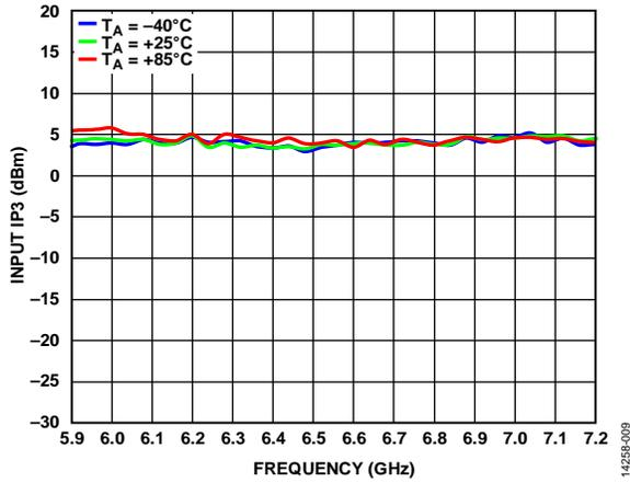
Figure 9. Input IP3 vs. Frequency for Various Temperatures
