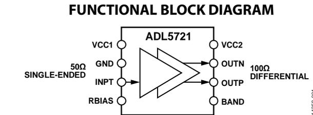
performance that, in the past, required more expensive three-five (III-V) compounds process technology to achieve. This LNA uses a band switch feature to allow the input P1dB and noise figure to trade off for optimum system performance.
