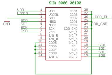
BMP280 shuttle board electrical layout
