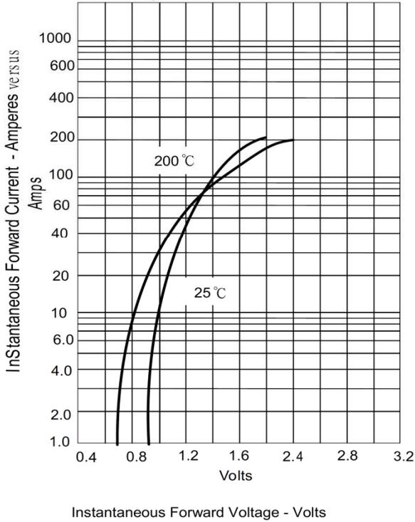
Figure .2- Forward Derating Curve
