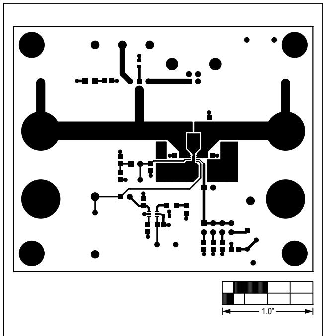
Figure 3. MAX14575A–MAX14575C EV Kit PCB Layout—Component Side
