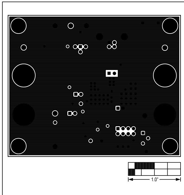
Figure 4. MAX14575A–MAX14575C EV Kit PCB Layout—Layer 2
