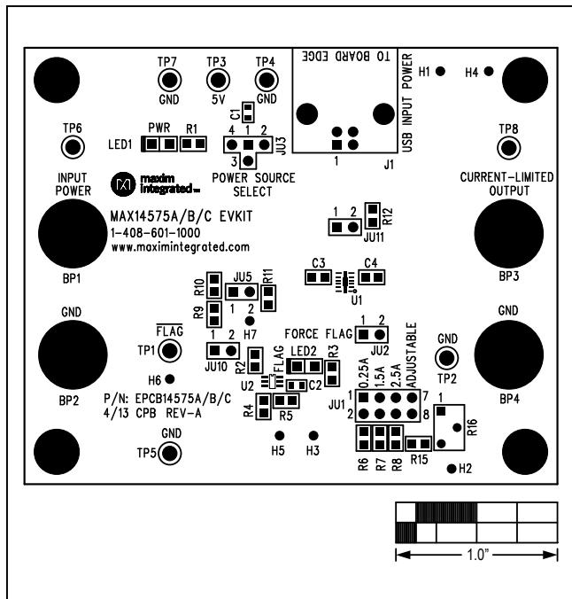
Figure 2. MAX14575A–MAX14575C EV Kit Component Placement Guide—Component Side
