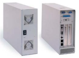
The physical appearance of the BBS-2003 resembles that of a power supply. However this small box houses the HS-6237 PCI-ISA Bus SBC that supports the Coppermine 800MHz CPU.
