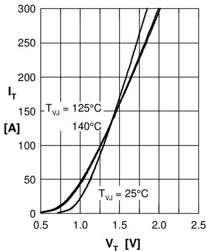
Fig. 1 Forward characteristics
