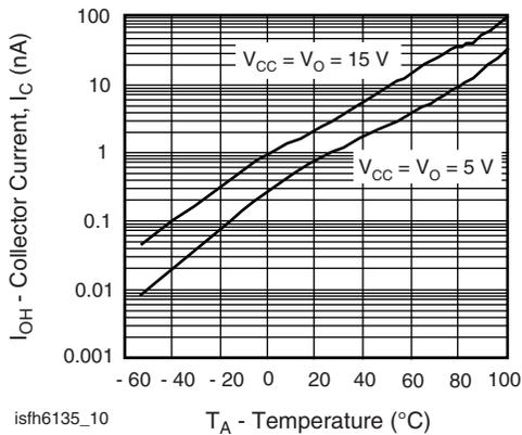
Fig. 9 - Logic High Output Current vs. Temperature
