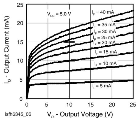
Fig. 6 - Output Current vs. Output Voltage
