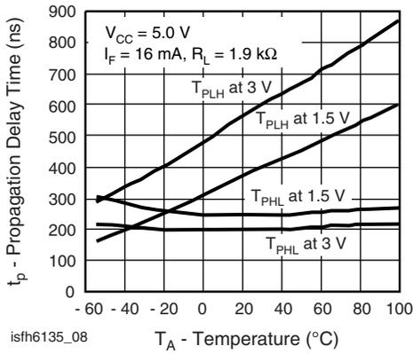
Fig. 8 - Propagation Delay vs. Ambient Temperature
