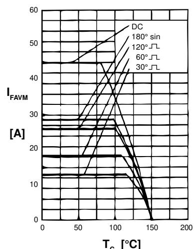
Fig. 3 Max. forward current
