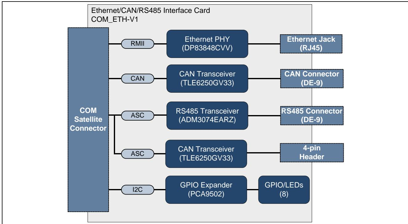
Figure 1 Block Diagram of the Ethernet/CAN/RS485 Interface Card
