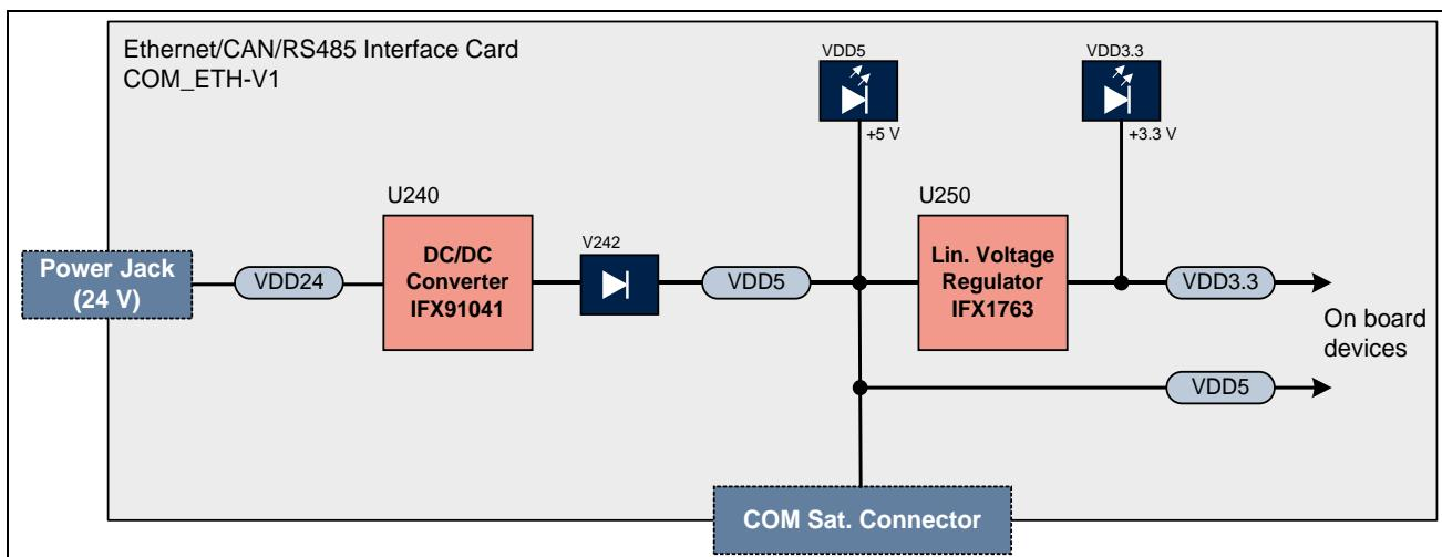
**Figure 6** Power Circuit
