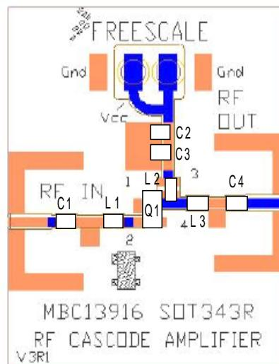
**Figure 11. 1.9 GHz Printed Circuit Board****Table 6. Electrical Characteristics**(V<sub>CC</sub> = 2.7 V, T<sub>A</sub> = 25°C, f<sub>RF</sub> = 1.9 GHz, Tested in Circuit Shown in [Figure 10](#), unless otherwise noted.)
