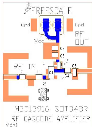
**Figure 9. 900 MHz Printed Circuit Board**
