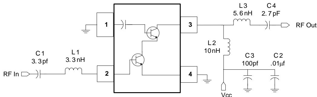
**Figure 10. 1.9 GHz Application Configuration Circuit**
