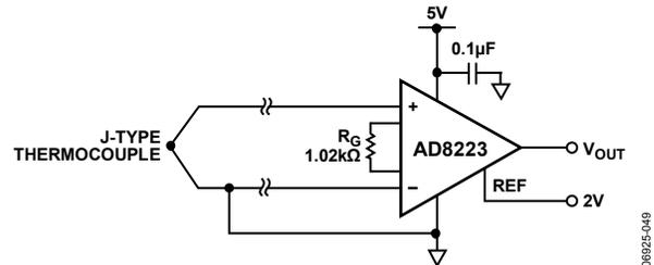
Figure 42. Amplifying Bipolar Signals with Low Common-Mode Voltage
