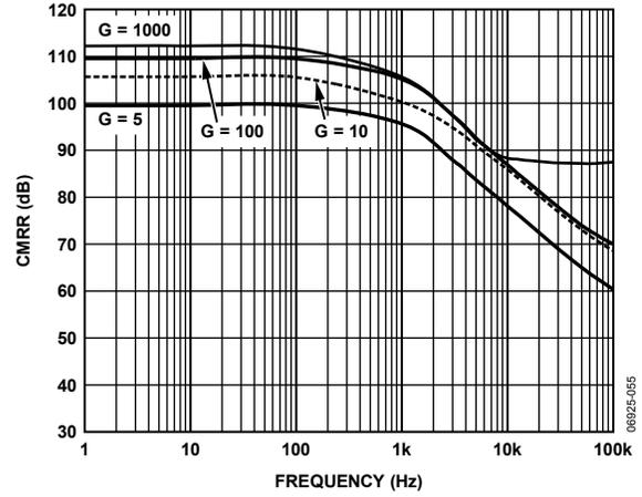
Figure 12. CMRR vs. Frequency,  $\pm V_S = \pm 12V$
