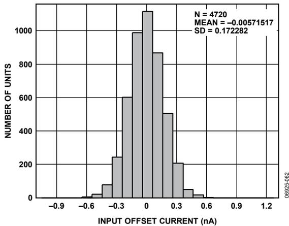
Figure 4. Typical Distribution of Input Offset Current
