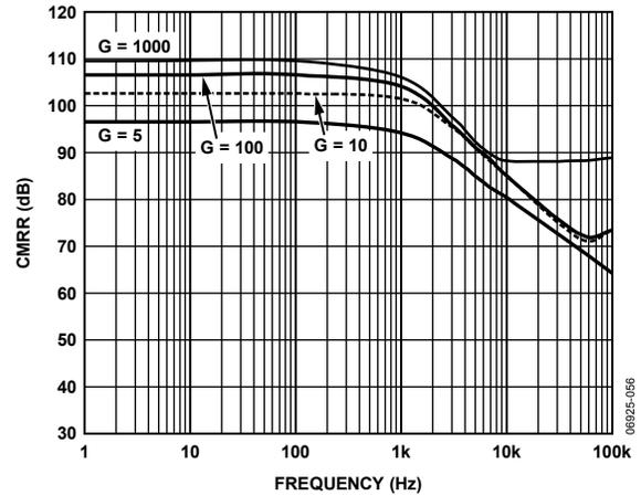
Figure 13. CMRR vs. Frequency,  $+V_S = +5V$
