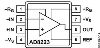
Figure 1. 8-Lead SOIC (R) and 8-Lead MSOP (RM) Packages
