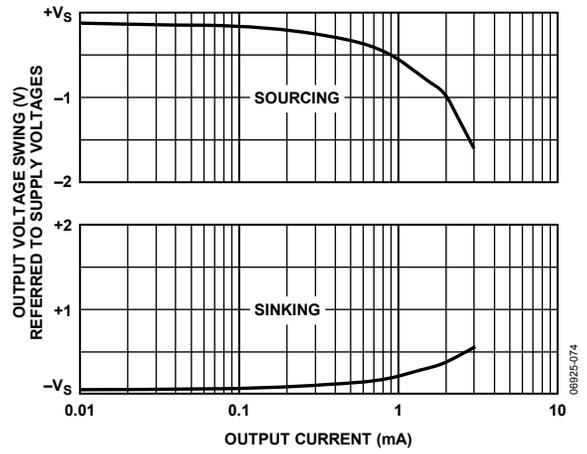
Figure 30. Output Voltage Swing vs. Output Current
