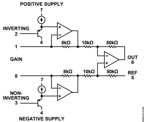
Figure 31. Simplified Schematic
