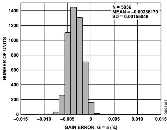
Figure 5. Typical Distribution for Gain Error ( $G = 5$ )
