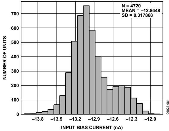
Figure 3. Typical Distribution of Input Bias Current
