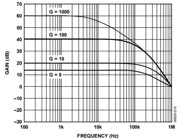
Figure 14. Gain vs. Frequency,  $\pm V_S = \pm 12V$
