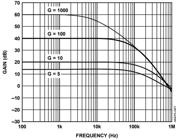
Figure 15. Gain vs. Frequency,  $+V_S = +5\text{ V}$
