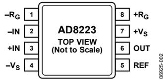
Figure 2. Pin Configuration
