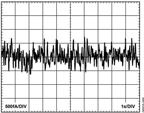
Figure 10. 0.1 Hz to 10 Hz Current Noise
