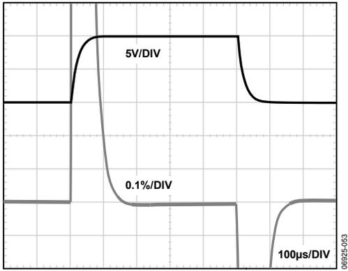
Figure 27. Large Signal Pulse Response,  $G = 1000$ ,  $C_L = 100$  pF
