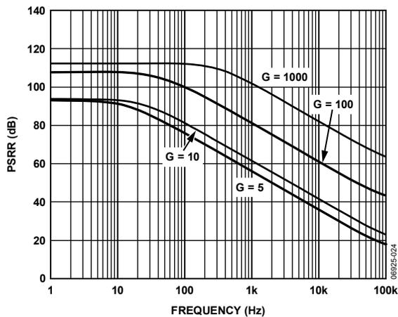
Figure 23. Positive PSRR vs. Frequency,  $+V_S = +5\text{ V}$
