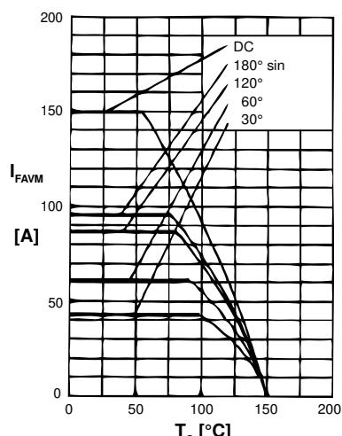
Fig. 3 Maximum forward current
