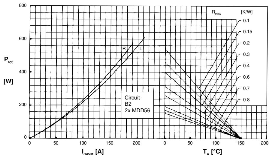
Fig. 6 Single phase rectifier bridge: Power dissipation versus direct output current
