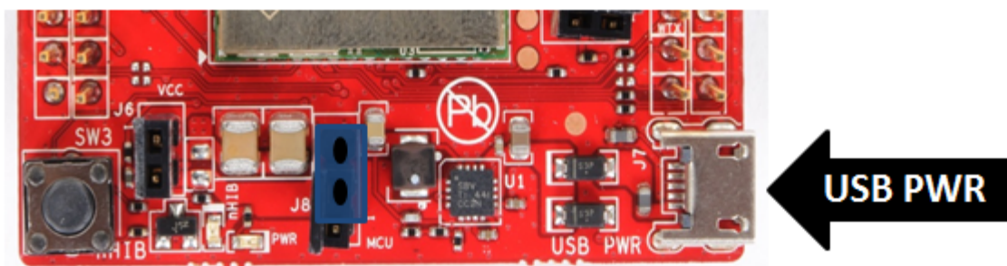
Figure 17. Jumper Settings When Used With LaunchPad
