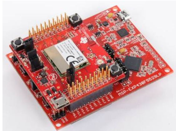
Figure 16. CC3100MODBOOST connected to MSP430F5529 LaunchPad
