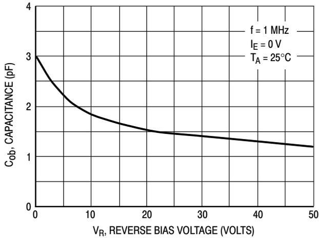
Figure 14. Output Capacitance
