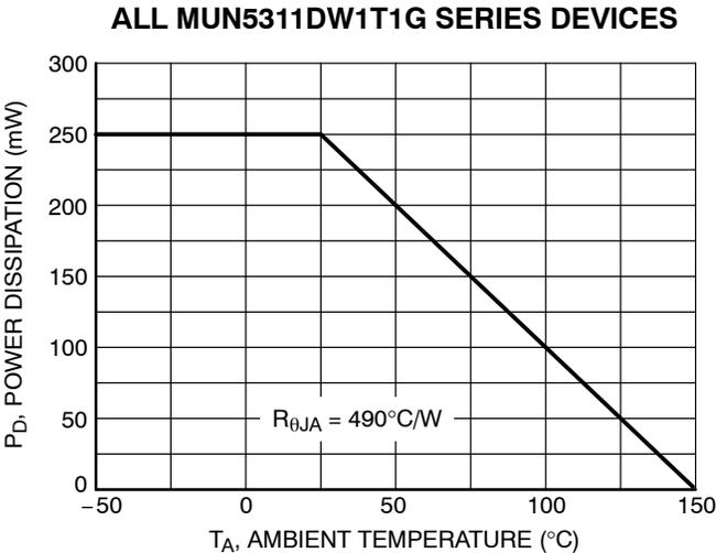
**Figure 1. Derating Curve**
