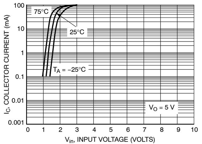
Figure 69. Output Current versus Input Voltage
