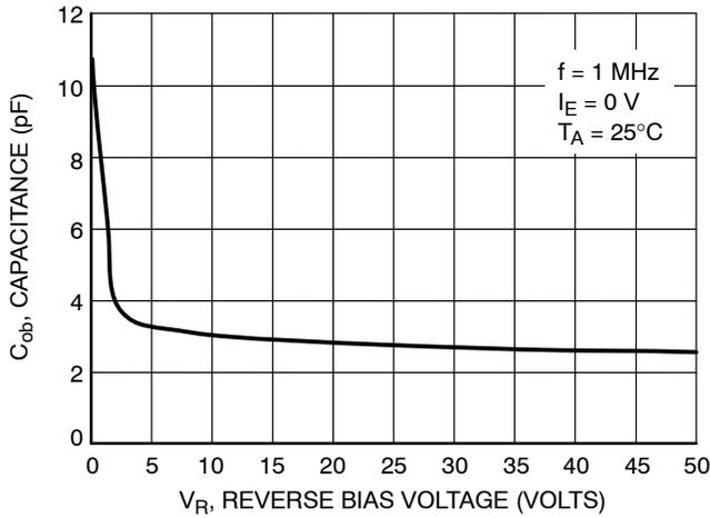
Figure 110. Output Capacitance
