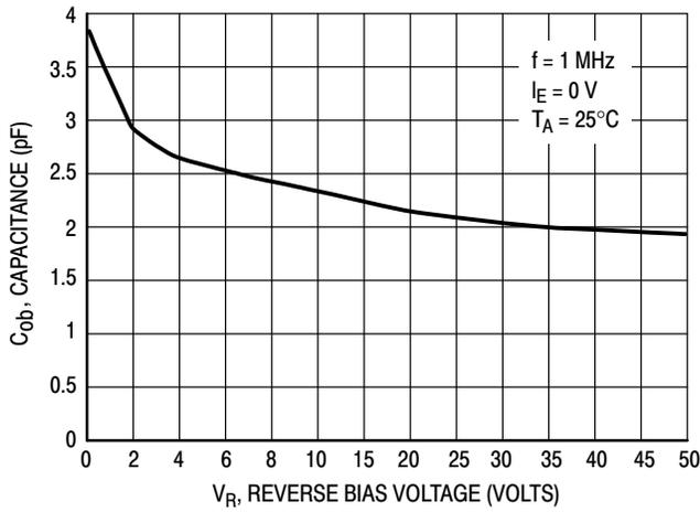
Figure 34. Output Capacitance
