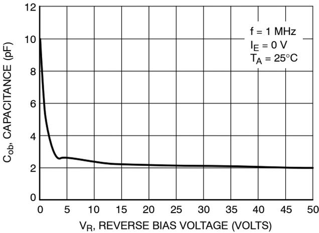
Figure 73. Output Capacitance
