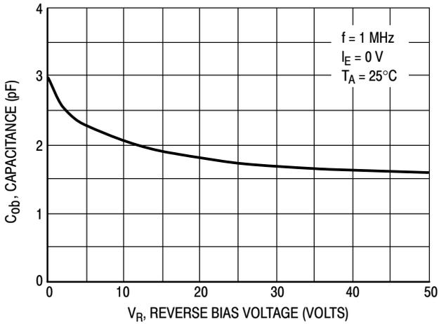
Figure 9. Output Capacitance
