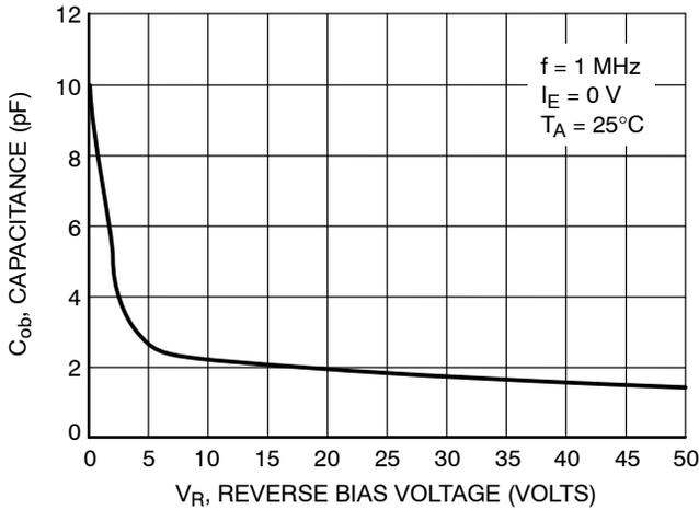
Figure 54. Output Capacitance
