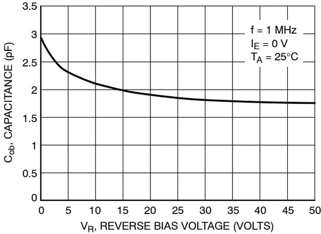
Figure 103. Output Capacitance
