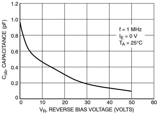
Figure 120. Output Capacitance
