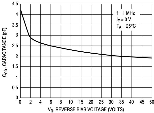
Figure 39. Output Capacitance
