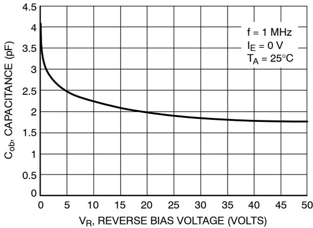
Figure 78. Output Capacitance
