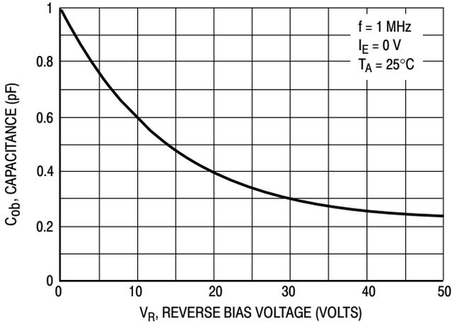
Figure 24. Output Capacitance
