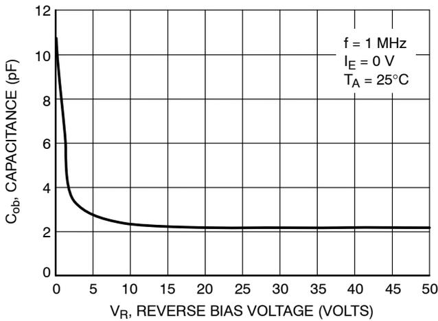
Figure 83. Output Capacitance
