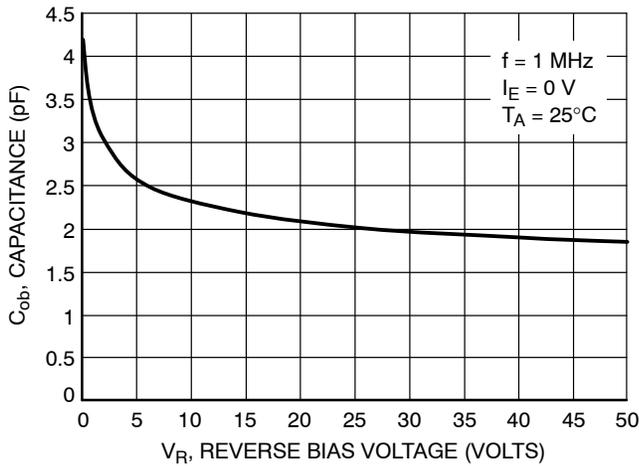
Figure 115. Output Capacitance
