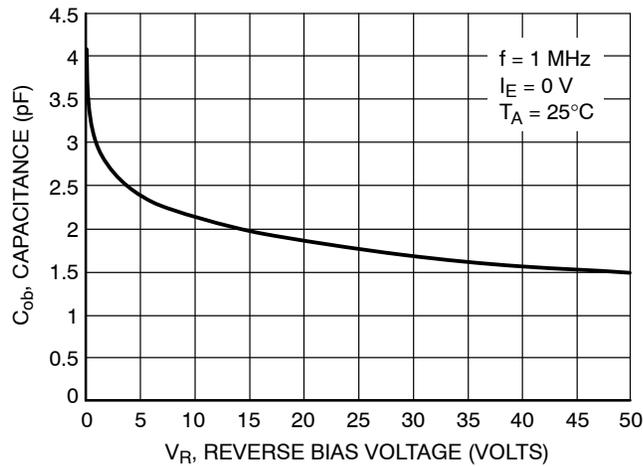
Figure 49. Output Capacitance
