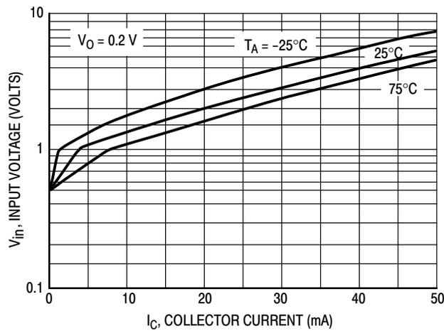
Figure 36. Input Voltage versus Output Current
