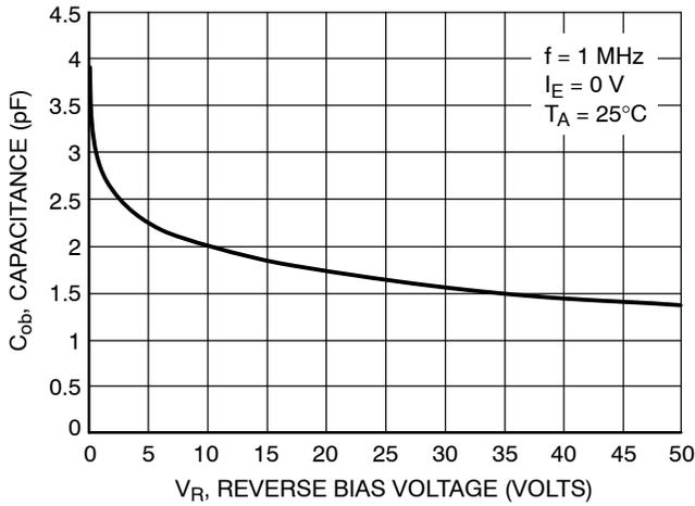
Figure 59. Output Capacitance
