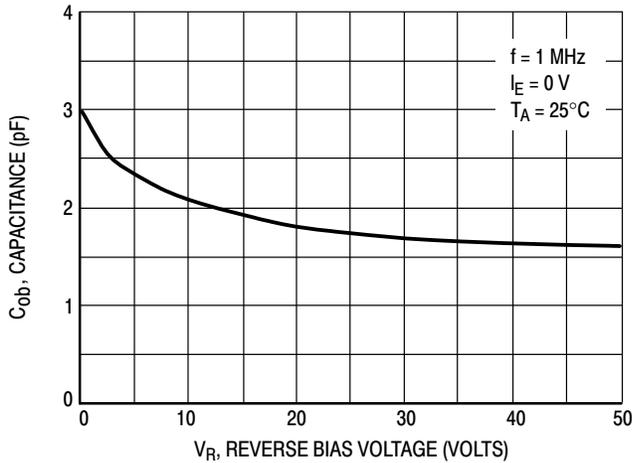
Figure 19. Output Capacitance
