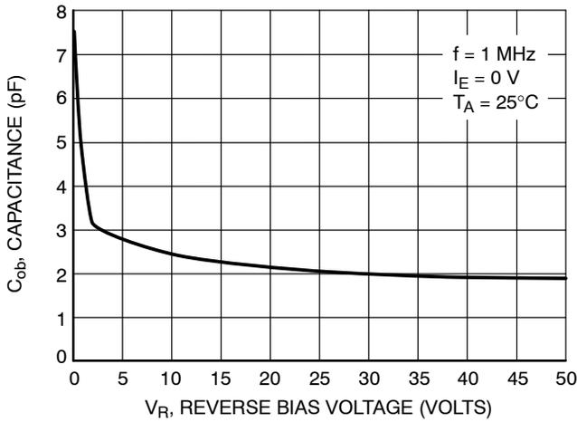
Figure 98. Output Capacitance
