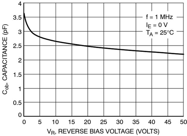
Figure 93. Output Capacitance
