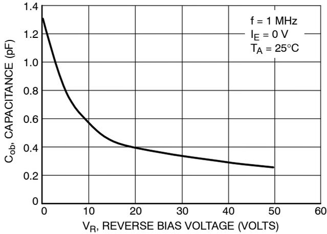
Figure 130. Output Capacitance
