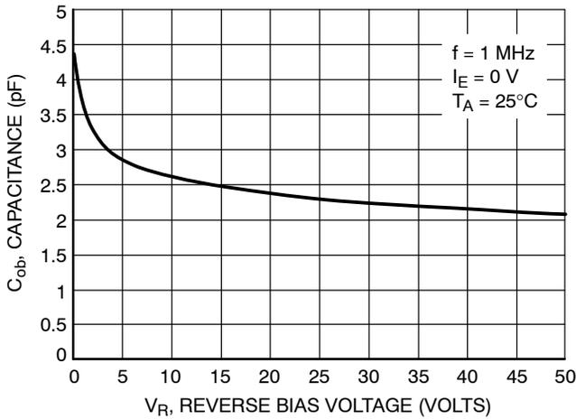
Figure 135. Output Capacitance
