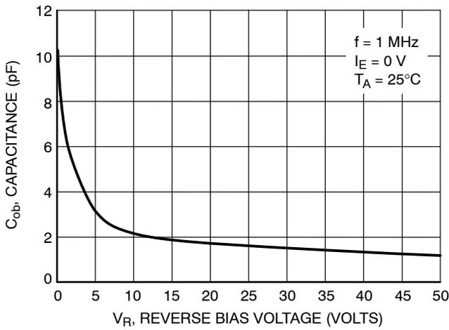
Figure 44. Output Capacitance
