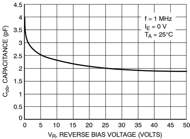
Figure 68. Output Capacitance
