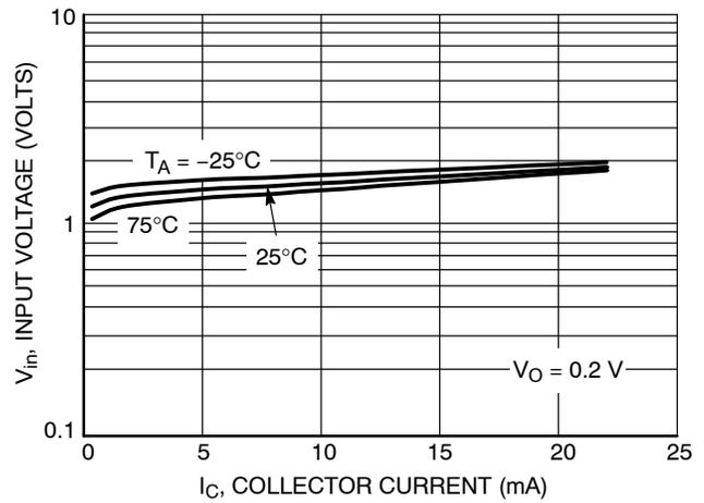
Figure 65. Input Voltage versus Output Current
