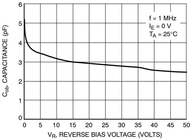
Figure 88. Output Capacitance
