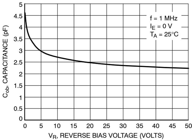
Figure 125. Output Capacitance
