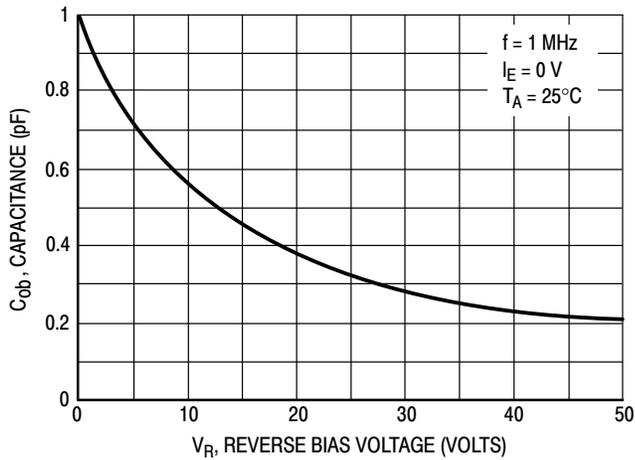
Figure 29. Output Capacitance
