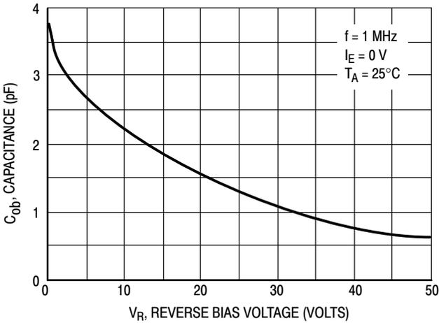
Figure 4. Output Capacitance
