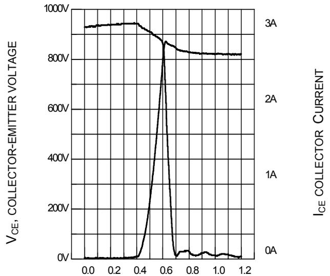
**Figure 20. Typical turn off behavior, hard switching**
