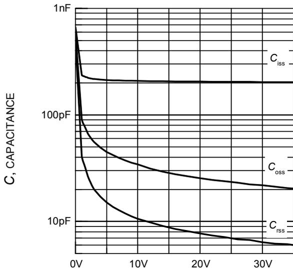
**Figure 18. Typical capacitance as a function of collector-emitter voltage**
