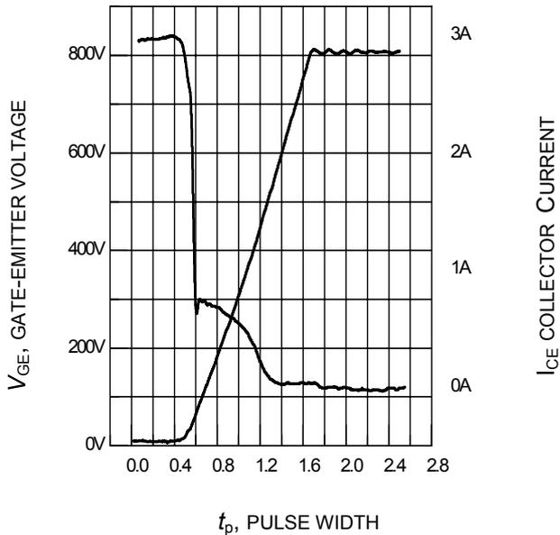
**Figure 21. Typical turn off behavior, soft switching**
