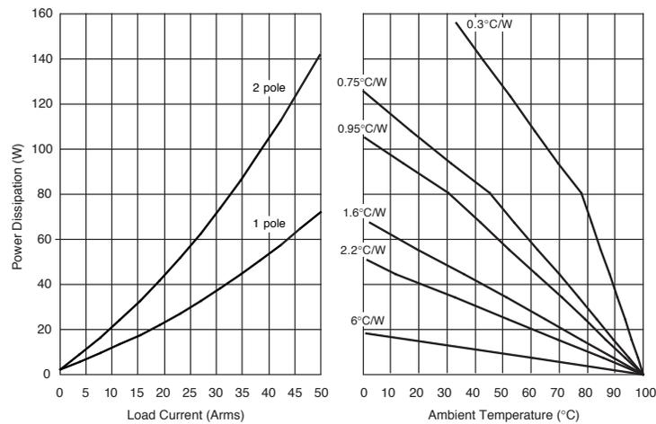
Figure 6c — SD48D50A and SD48D50A2 output current
