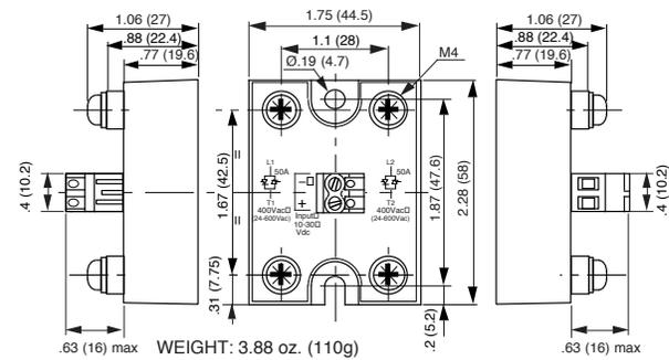
Figure 2d — SD48D50A; dimensions in inches (mm)
