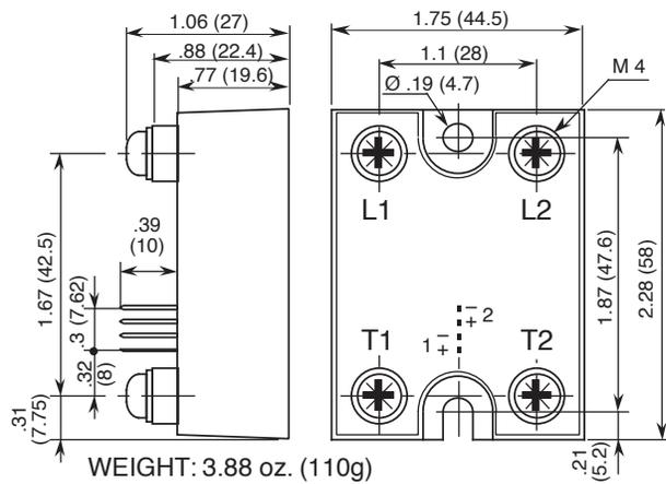
Figure 2b — SD24R50; dimensions in inches (mm)
