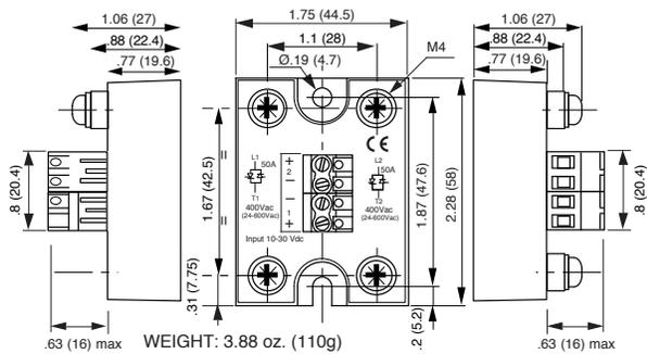
Figure 2e — SD48D50A2; dimensions in inches (mm)
