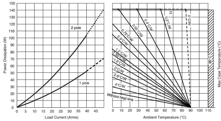
Figure 6a — SD24 50A relays output current
