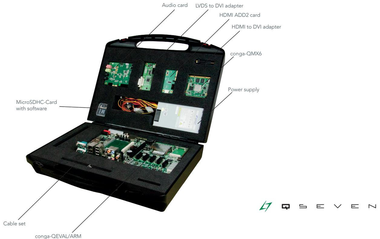
This complete kit provides the ability to start evaluating Qseven® ARM modules immediately.
