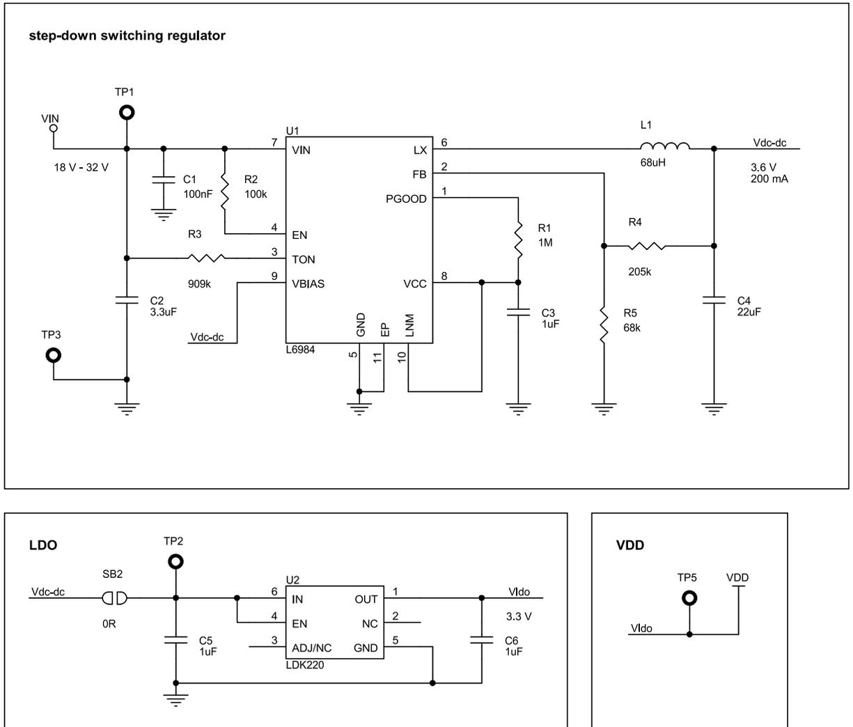
**Figure 7. Schematic - STEVAL-IDP005V1 (6 of 7)**
