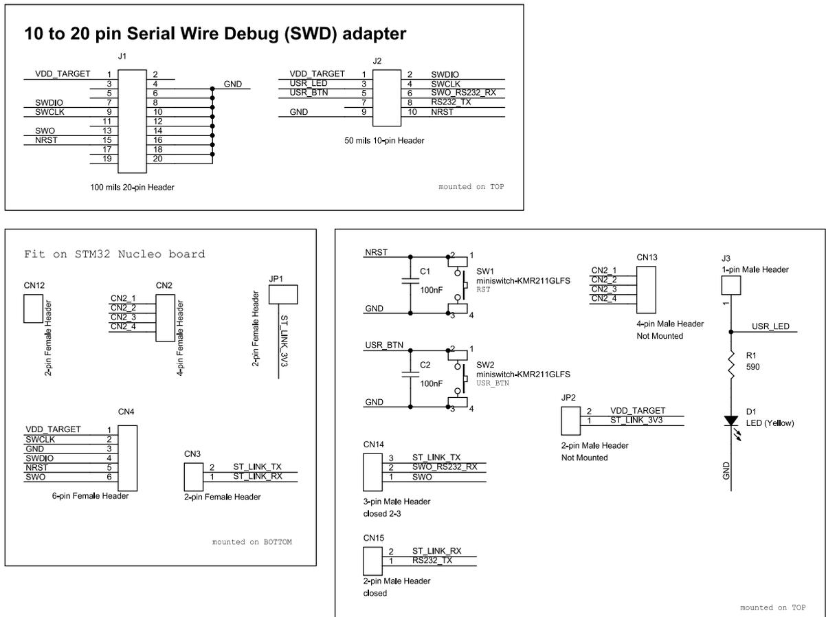
Figure 2. Schematic - STEVAL-IDP005V1 (1 of 7)
