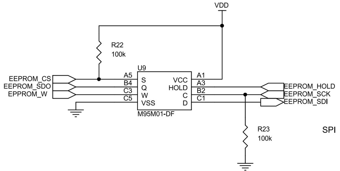
**Figure 6. Schematic - STEVAL-IDP005V1 (5 of 7)**
