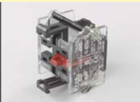
Contact block, screw terminal, slow-make (positive-break) with silver forced opening contacts
