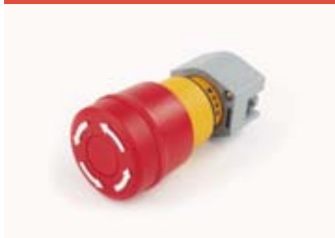
Emergency-stop, twist release, 37mm diameter, foolproof to EN 60947-5-1 and EN 418, use slow-make switching elements
