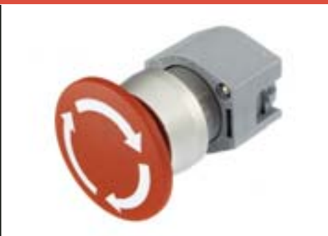
Emergency-stop, twist release, mushroom head, 40mm diameter, use slow-make switching elements
