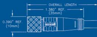
STRAIGHT FEMALE SINGLE ENDED THREADED COUPLING
